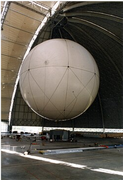
The CargoLifter CL75 AirCrane, a cargo-lift mechanism using a balloon filled with helium, inside the CargoLifter hangar ✎
